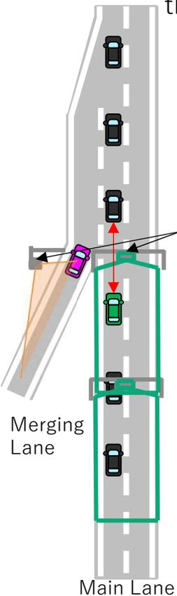
**Road-vehicle communication equipment & Vehicle monitoring sensor**
