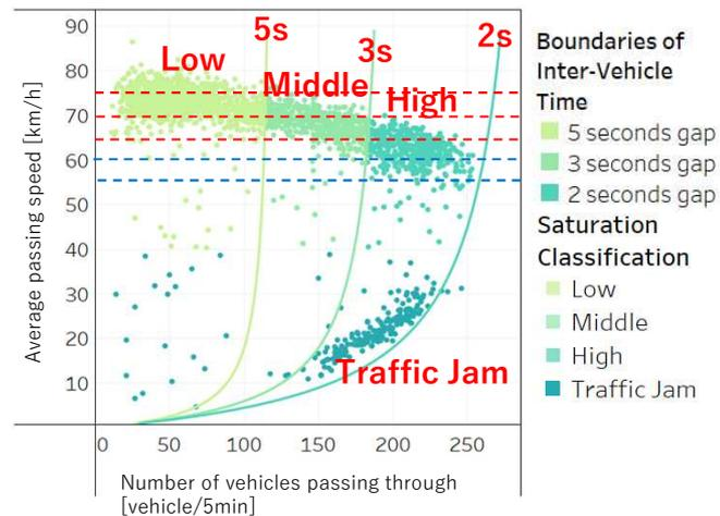
Parameter combination during simulation (assistant area design from Q-V diagram)
