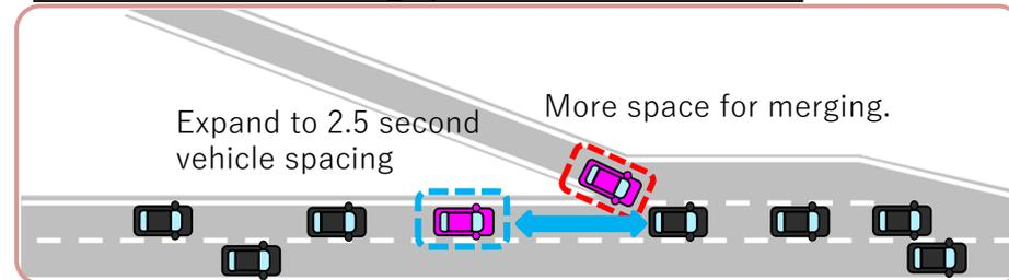
In addition to side-by-side avoidance with main lane vehicles, the Day3 system allows merging into a larger gap between vehicles.
