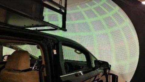
Constructed a spherical wide-angle screen that allowed evaluation of mono camera, and **completed evaluation of consistency with the actual mono camera**
