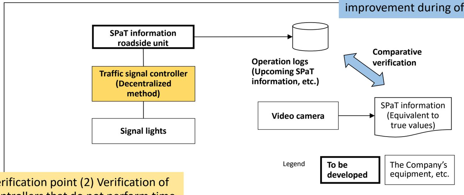
Verification point (2) Verification of controllers that do not perform time synchronization
