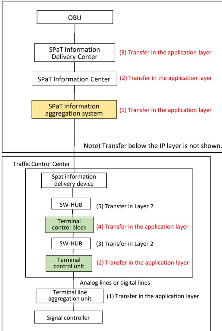
Verification point (1) The cause of the communication delay is assumed to be the transfer in the application layer.
