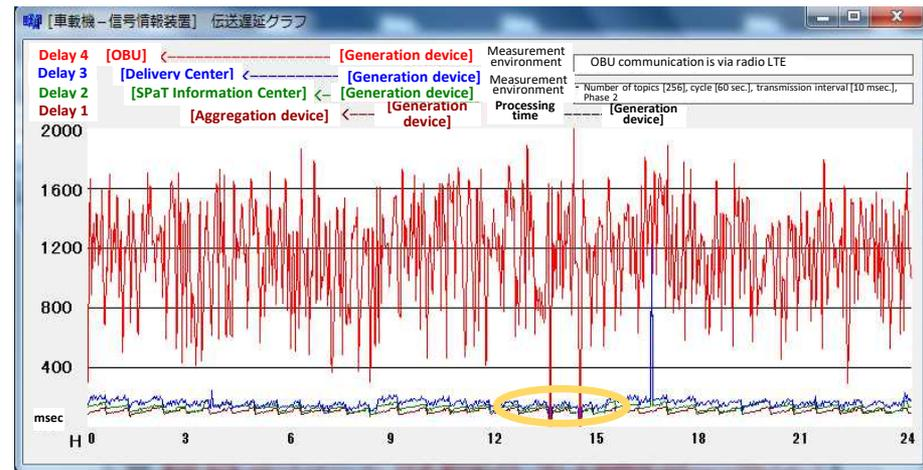
Continuous operation without MQTT-PING
