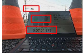
Recognition error = Time when the traffic light color changed – Time when the traffic light color indicated by OBU changed
