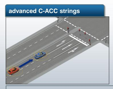
Based on intended maneuver at next intersection, vehicles assess the convenience of building small strings, and keep them using exchanged trajectory for lateral control
