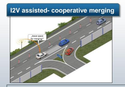
Infra suggest info to coordinate right of way in a way to optimise the overall traffic flow
