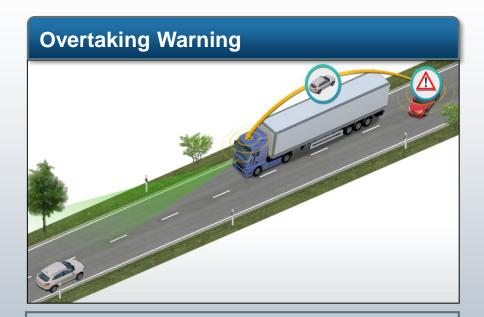
Overtaking car analyses the rx info and warn the driver if necessary
