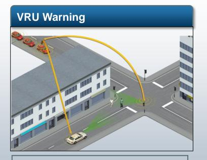
Turning car analyses the rx info and warns the driver if necessary
