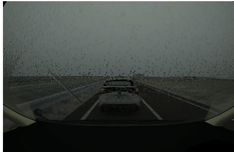
Rain adhesion model on windshield
