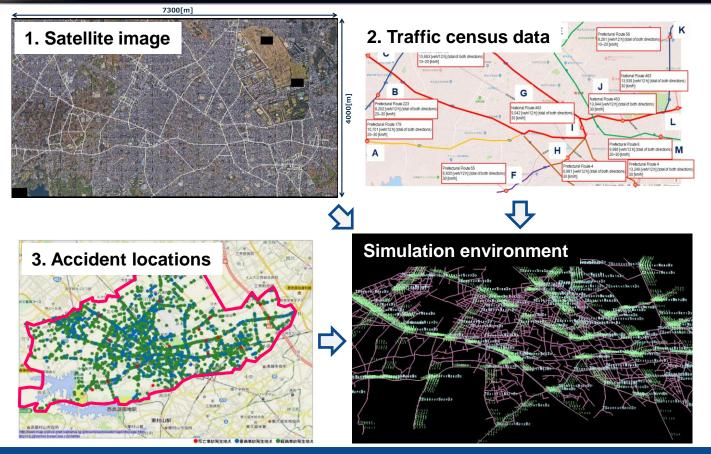
Build the main road network in each model city, and reproduce the traffic flow and traffic accidents
