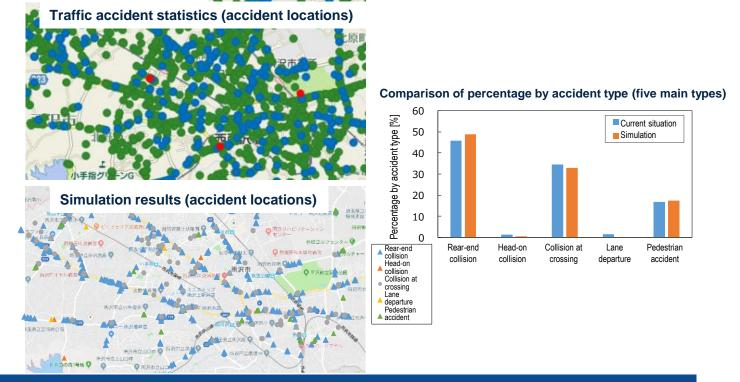
Confirmation of validity based on comparison between the accident locations in the traffic accident statistics (2015–2017) and the simulation results
