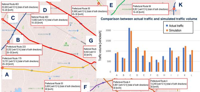
We confirmed that the traffic flow, which reflected the characteristics of traffic volume of 12 hours during the daytime at the main points within the scope of the simulation, was reproduced.
