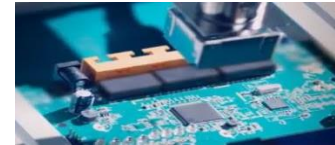
Removal of chips from ECUs
