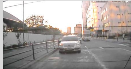
↓ The traffic signal arrow turned yellow, so the test vehicle rapidly braked. The following vehicle intended to turn right, so it accelerated.
