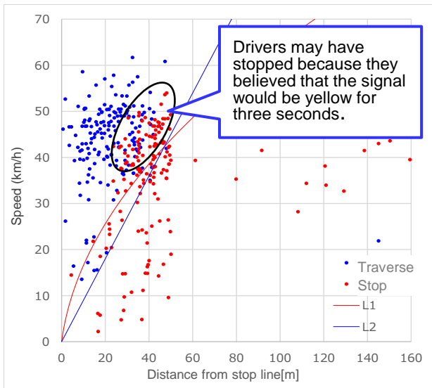
Fig.: Distribution of intersection traversal decisions during manual driving
