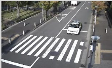
The vehicle detects the crosswalk pedestrian and suddenly decelerates (0.38G). The vehicle crosses the stop line by a large amount and draws near the pedestrian.
