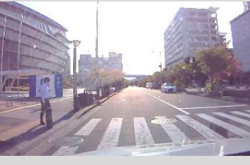
The vehicle detects the crosswalk pedestrian and suddenly decelerates (0.38G). The vehicle crosses the stop line by a large amount and draws near the pedestrian.
