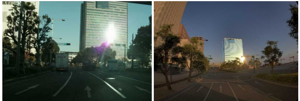
Example of verification for failure scene of traffic light detection under backlight of reflected sunlight (Left: real, Right: simulated image)
