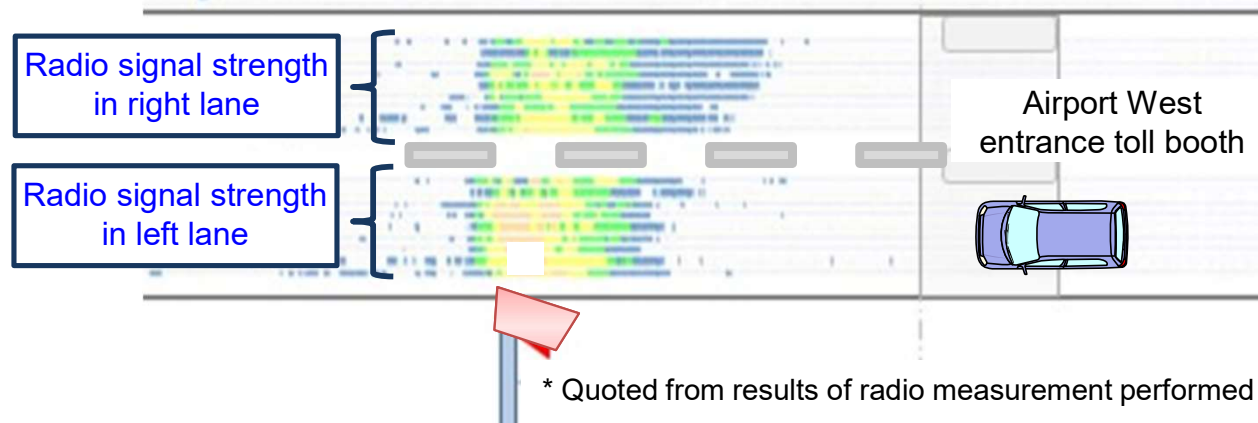
Radio signal strength at antenna behind toll booth (actual measurement values: details)
