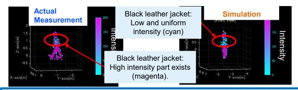
Although black leather jacket have specular components, they are not reproduced in the model ⇒ Candidate of difference factor
