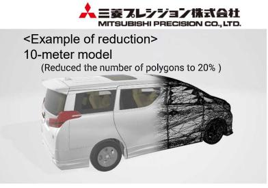
×1 It is possible to set thresholds/conditions such as number of polygons, direction of normal before and after reduction, preservation of holes/boundaries, priority of blunting angle, etc.
