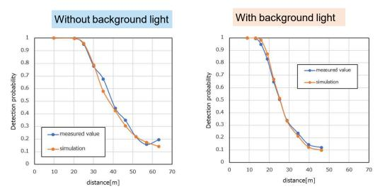
Confirm consistency of ranging limit (detection probability) by both conditions without background light and with background light.
