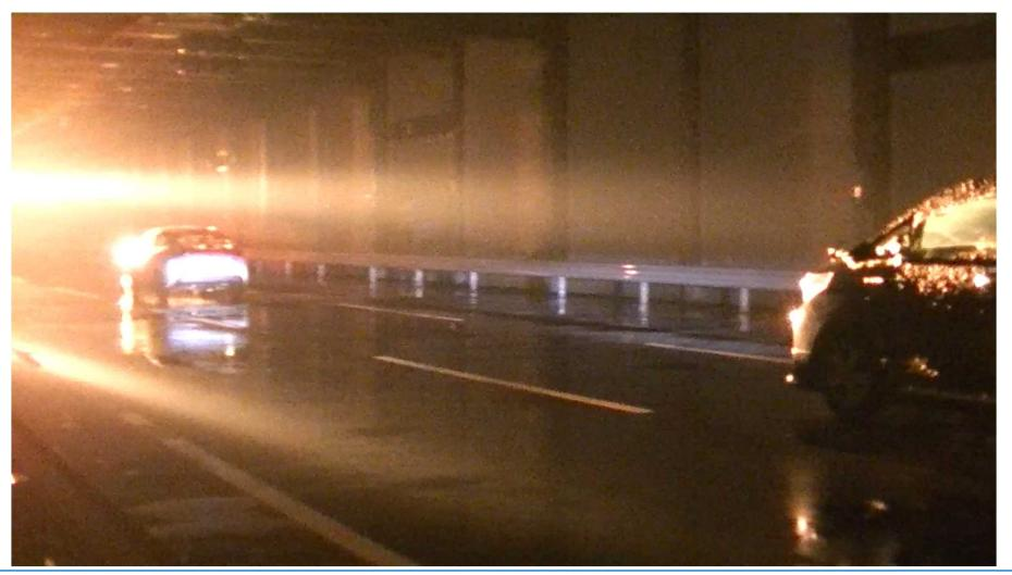
We conducted a factor study of modeling based on the NIED\* rainfall test, and we were able to measure the phenomenon and the factors of malfunction peculiar to rainfall
