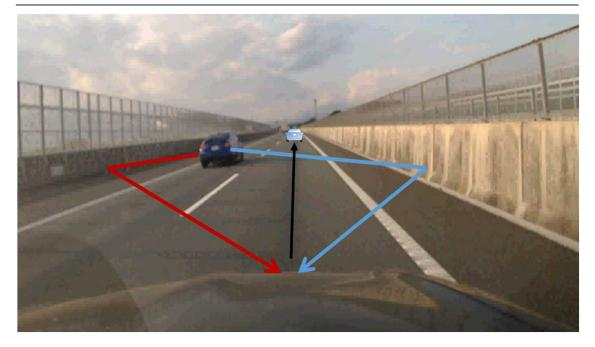
False recognition of the presence of the preceding vehicle due to multipath synthesis Multipath case 2 of Radar
