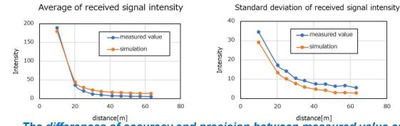
The differences of accuracy and precision between measured value and simulation are small, and the measured value tends to be higher than simulation.
