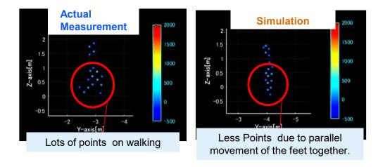
Large difference in the shape of the lower half of the target between actual measurement and simulation ⇒ Candidate of difference factor
