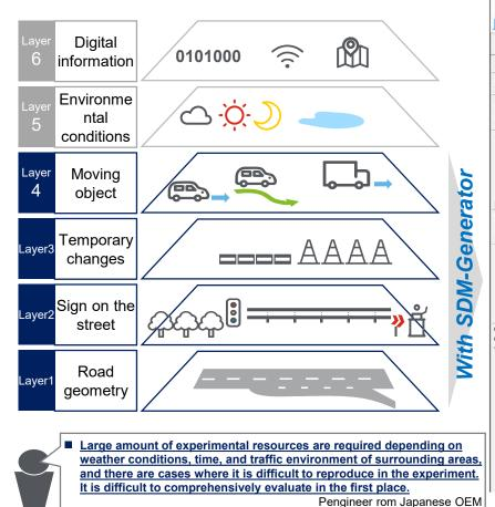
Creation of traffic environment models using SDM-generators
