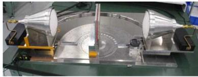
Measurement of dielectric constant and magnetic permeability by free space method
