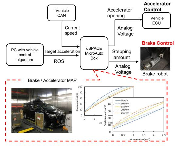
Configuration of automatic brake control system
