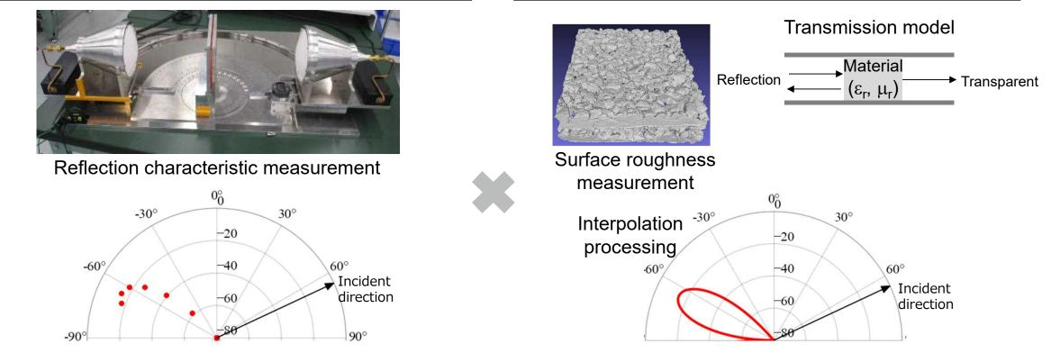
Measure surface and material characteristics as well as material reflection characteristics Create reflection data for interpolation processing of the theoretical formulas
