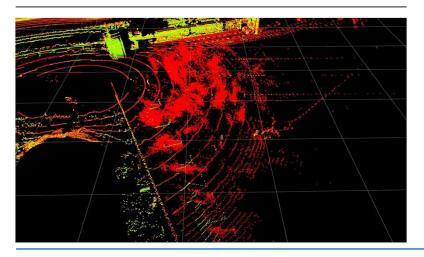
Effect of raindrops on the front surface of the sensor : False Negative
