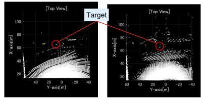
Differences in the shape of the target point cloud ⇒Possible cause of difference Differences in the shape of ambient point cloud of the target ⇒ Investigation of the effect of point cloud around the target (next page)
