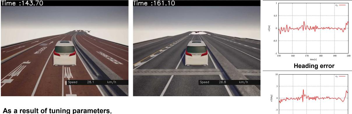
Travel with accuracy within 25 cm of lateral error and within 4 ° of heading error with respect to the center of the own lane
