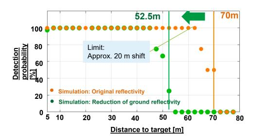
Ground reflectivity differences around the target significantly reduce the target's detection limit for long distance.
