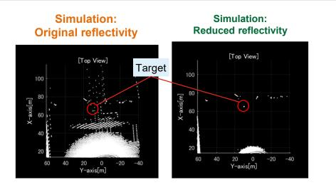
Differences in the detection limit of distant targets due to differences in point cloud around the target
