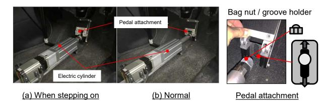
Brake robot unit to reproduce the actual driver's movement
