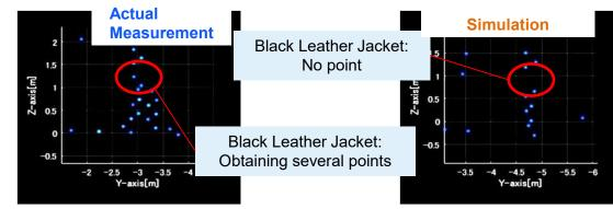
Difference in intensity of a black leather jacket (distance to target: 8 m)
