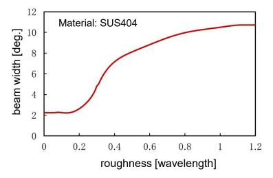
Example) Relationship between surface roughness and reflected beam width
