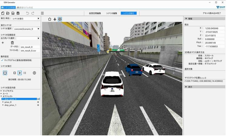
\*: <u>S</u>pace <u>D</u>esign <u>M</u>odel Source : MITSUBISHI PRECISION CO., LTD. It is possible to assemble any traffic environment such as road shape, placement of traffic participants, movement setting and also environmental factors such as rain and backlight.
