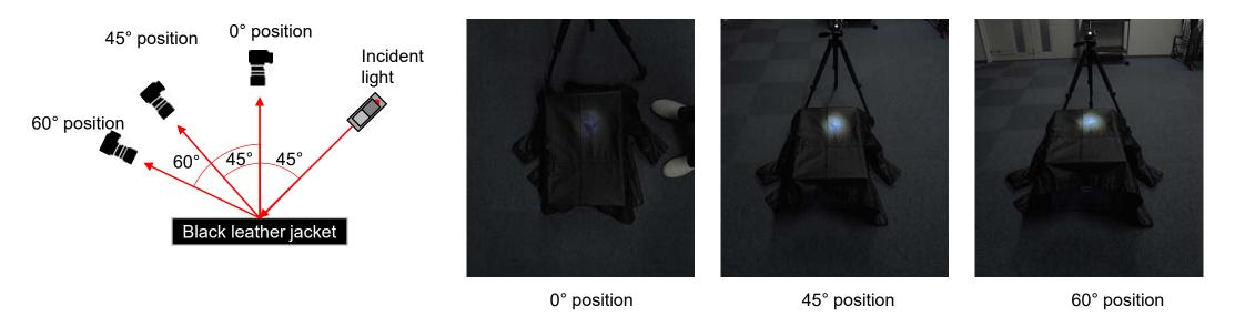
Confirm that the black leather jacket contains a specular reflection component significantly larger than the diffuse reflection component.
