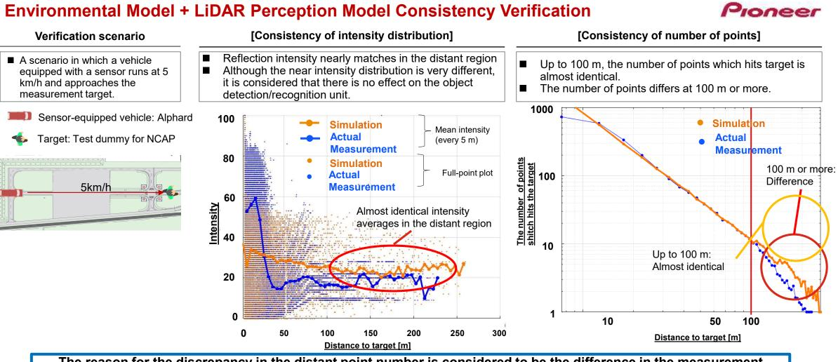
The reason for the discrepancy in the distant point number is considered to be the difference in the measurement distance limit of LiDAR.
