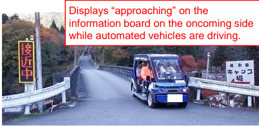
Advance notice of approach by automated vehicle on information board
