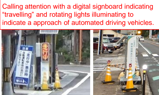
Preliminary notice of automated driving vehicle approaching with digital signboard and rotating lights
