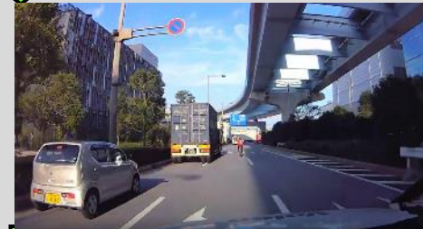
It detected a sports-type bicycle in front and applied sudden braking (approx. -0.44G).
