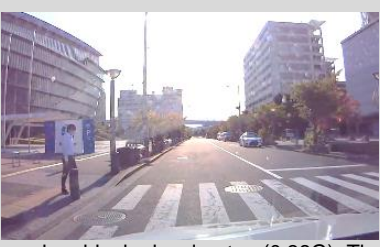
↓ The vehicle detects the crosswalk pedestrian and suddenly decelerates (0.38G). The vehicle crosses the stop line by a large amount and draws near the pedestrian.
