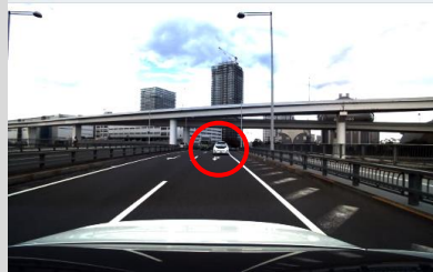
The test vehicle decelerated due to a red traffic light (-0.2G) (Deceleration start point: 82 meters ahead of stop line)
