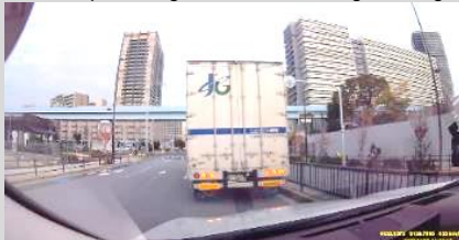
The test vehicle entered the right turn lane, rapidly approached the stopped large vehicle, and rapidly braked (-0.56G)
