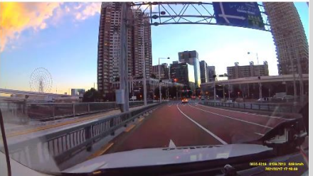
➡ The test vehicle decelerated somewhat suddenly due to a red traffic light (-0.24G) (Deceleration start point: 48 meters ahead of stop line)
