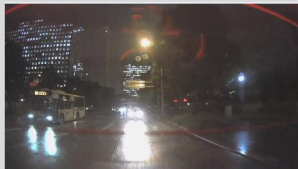
Infrastructure information was received and the test vehicle began preliminary deceleration in advance (98 meters before reaching the stop line)
