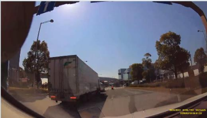
The test vehicle detected a traffic light and a preceding vehicle (motorcycle) and began decelerating (72 meters before the stop line)
