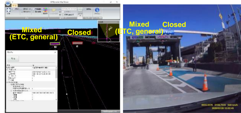
ETC gate passing support information (comparison of viewer display and test video data recording device image) February 28, 2020, 12:02:49
