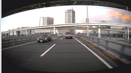
➡ The test vehicle decelerated somewhat suddenly due to a red traffic light (-0.24G) (Deceleration start point: 48 meters ahead of stop line)
