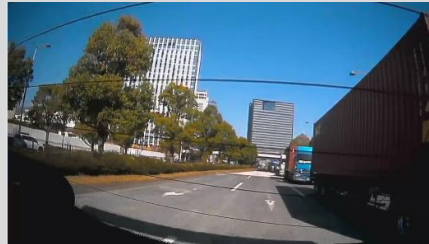
The test vehicle detected a traffic light and a preceding vehicle (motorcycle) and began decelerating (72 meters before the stop line)
