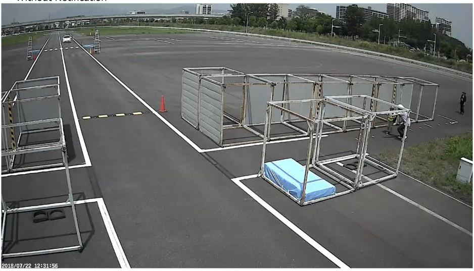
2)Intersection with poor visibility (30km/h) Pedestrian Verification
