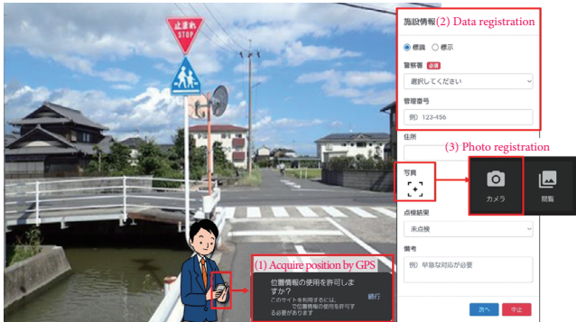
Fig.8: Image of registering road signs/markings on smartphone device
