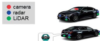
Outline of Honda Legend automated driving system *Provided by Honda Motor Co., Ltd.
