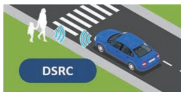
Fig. 7 Vehicle-to-pedestrian communication using DSRC
