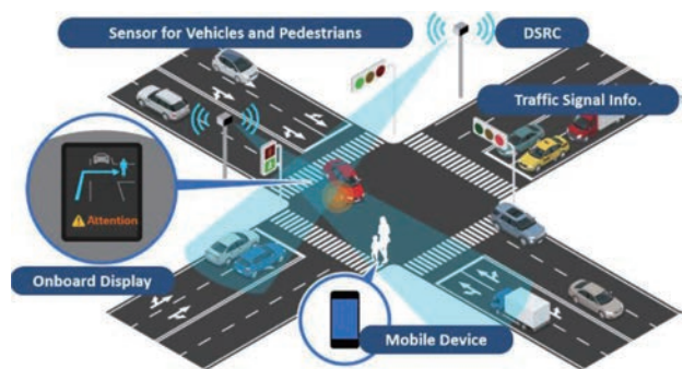
Fig. 9 ITS information services at an intersection
