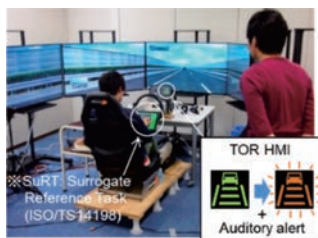
Fig. 3 The driving simulator at the University of Tsukuba used for the Task A experiments.
