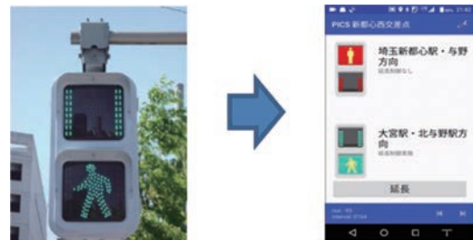
Figure 4 Pedestrian signal lamp (indication of time passed)
