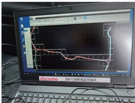
Fig. 7 Lane-level traffic flow field check using SIP Dynamic Map Viewer
