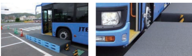
Fig. 4 Scenes of precise docking control
