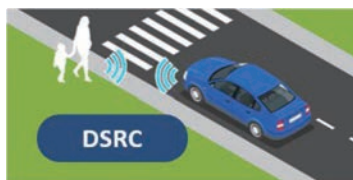
Fig. 7 Vehicle-to-pedestrian communication using DSRC
