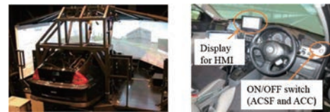
Fig. 5 External view and driver's seat of DS
