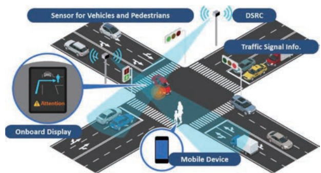
Fig. 9 ITS information services at an intersection
