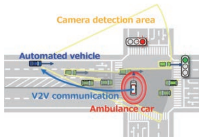
Fig. 3 Emergency vehicle recognition support model using V2V communication
