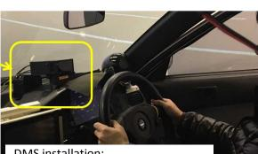
DMS installation: -Distance to face: 650mm -Location: Upper left of meter hood
