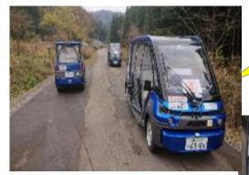
One remote monitoring and operation person operates three unmanned automated driving vehicles
