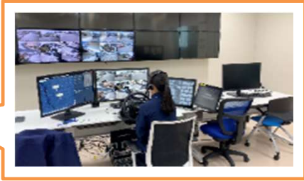
[Monitoring and control] Taking advantages of Local 5G, such as hi-speed and large capacity, Operator monitors or controls automated driving bus with Full HD video
