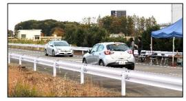
Small deceleration (25km/h  $\rightarrow$ 15km/h, Ave. -1.03m/s<sup>2</sup>) Large deceleration (25km/h  $\rightarrow$ 10km/h, Ave. -1.35m/s<sup>2</sup>)
