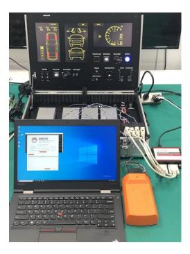
Fig1. IDSs provided by Arilou are connected to PASTA and running. addition to IDS (Fig3), both companies also provided monitoring environments.
