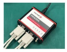
Fig2. Vector VN1630A + CANPiggy × 2 The above is controlled by CANoe.
