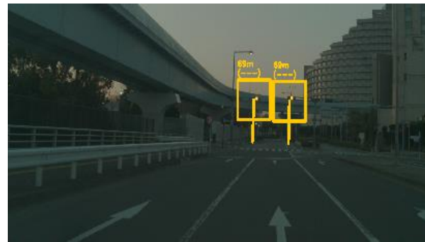
Recognize “yellow” 40[m] before stop line (Distance to traffic light : 69m)
