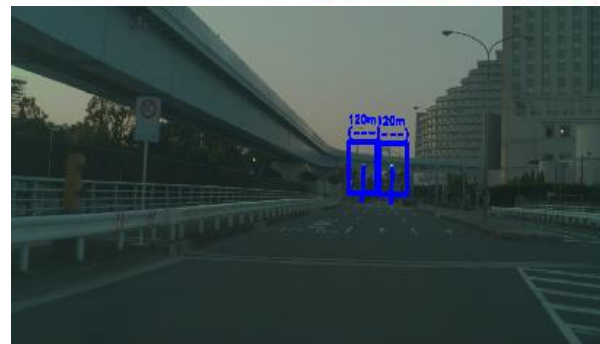
Approaching intersection as recognized “blue” (Distance to traffic light: 120[m])
