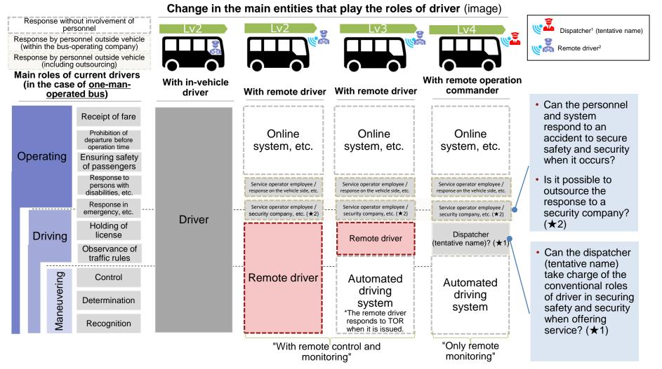
1. Dispetcher (tentative name): This person remotely operates an Lv4 vehicle when it has broken down or the like, if necessary.
