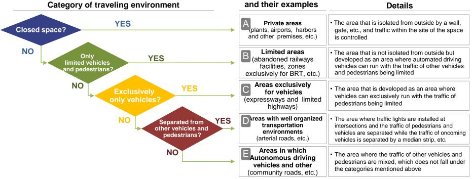
\* "A to E" only show basic types and do not necessarily indicate the order of difficulty because actual driving environment consists of various conditions such as those shown as complementary elements.
