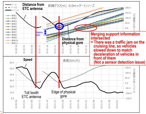
Merging support information received and vehicle merging into cruising line vehicle gap
