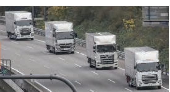
FOT of 4 brands truck CACC+LKA. Dec, 2018 (Time to Collision: 1.6 sec 80km/h)
