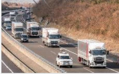
FOT of 4 brands truck CACC. Jan, 2018 (Time to Collision: 1.6 sec 80km/h)
