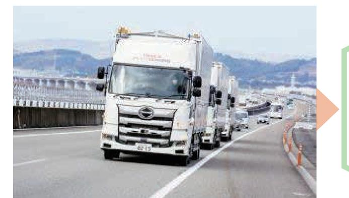
FOT of CACC+ Lead Truck Following System. Jan-Feb, 2018 (Time to Collision: 0.5sec 70km/h)
