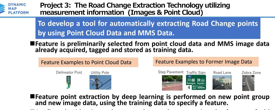
Confirm the identity and extract changes by comparing the feature of old data and newly extracted feature of the area of interest.
