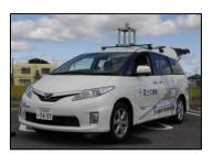
Uses High-precision 3D map and LiDAR.
