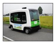
Uses GPS and IMU.
